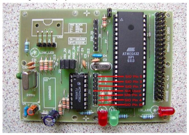
Locate on SIO2IDE motherboard connector named **SIO\_IO** (it is located next to chip U3). Use this connector to connect your SIO2IDE to Atari. Build you cable according to diagram provided in User Manual and in this guide.
